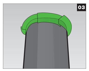
Apply Rissan around circular parts in layers
